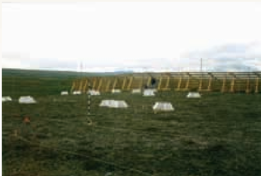
Figure 8. Snowfence experiment within the Toolik Lake Grid, summer view showing fence, snow-depth monitoring stakes, and small open-top greenhouses.
