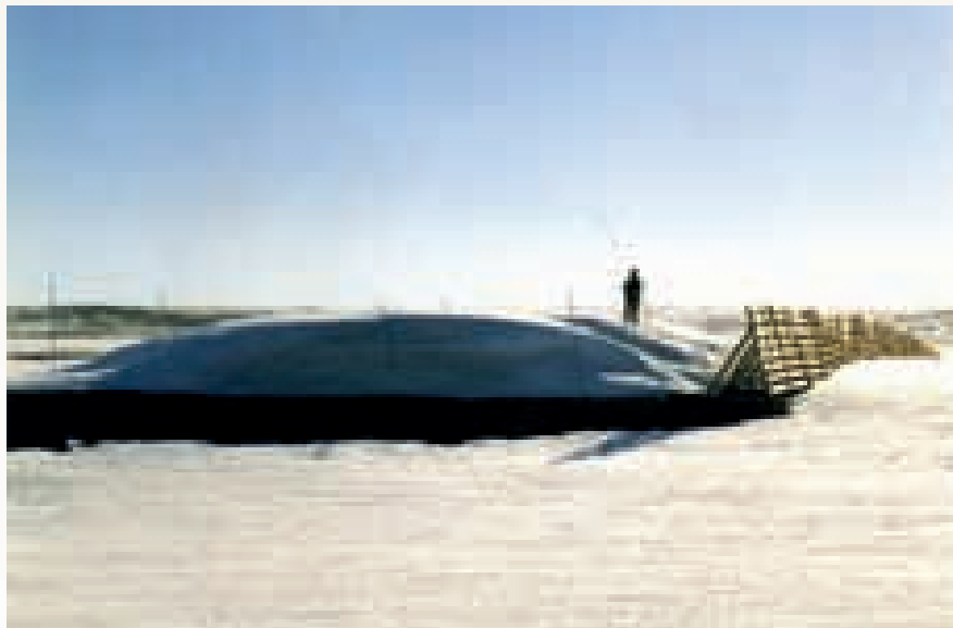
Figure 9. Winter view of snowfence experimental area showing the drift that has built up behind the fence. Tall stakes are the same as striped stakes in Figure 8.
