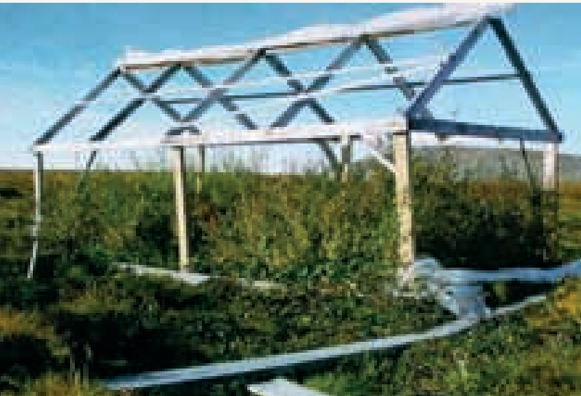
Figure 7. Experimental greenhouse with the side and top opened to show enhanced growth due to added warmth. Pre-treatment shrubs were same height as vegetation in the foreground.
